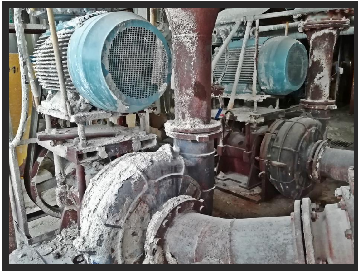
ETİ MADEN BORON WORKS (KIRKA) SEP GSP-VX & GSP MK SERIES HEAVY DUTY MINERAL/SLURRY PUMPS (BORON WORKS)
